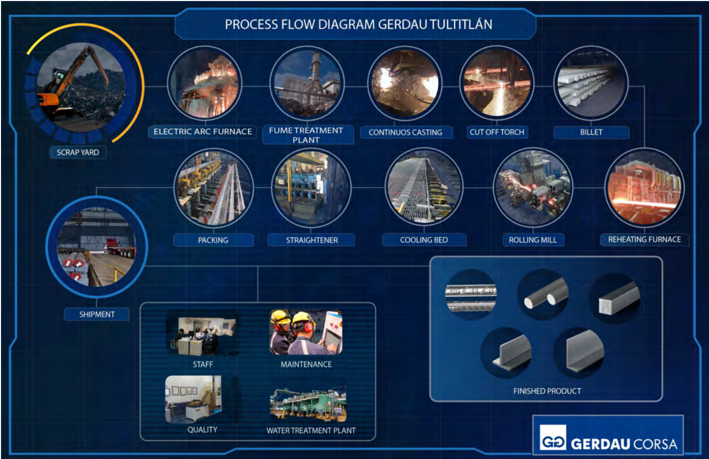
Figure. 1. Flow diagram of steel rebar manufactured from steel scrap
